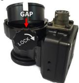
spotting device and turn the lock screw tight.
